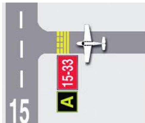
Pilots also use signs to figure out where they are and where they are going. **Destination signs** (black on yellow) show direction to listed destination. **Taxiway directional signs** show the direction of a taxiway, for example when coming out of an intersection. **Taxiway location signs** (yellow on black) identify which taxiway you are on.
