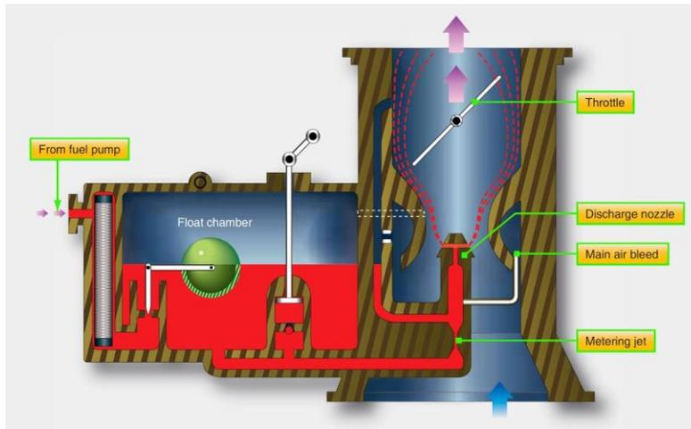
A disadvantage of carbureted-engines is **carburetor icing**, likely to form when [REDACTED]. The first indication for the pilot is a loss of RPM. To correct, apply carburetor heat and expect a further RPM decrease (richer mixture, more on that in a bit) followed by an increase as the ice melts.
