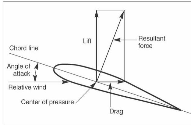
The **critical angle of attack** is the angle at which the wing will [redacted]. This angle is independent of factors like weight and loading.
