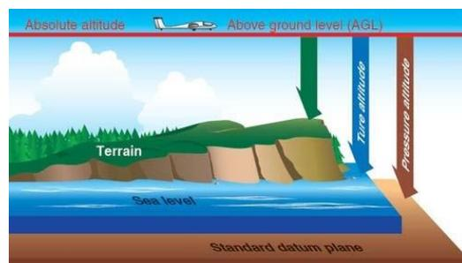
We adjust the altimeter setting on the ground  so that indicated altitude is approximately equal to true altitude.
