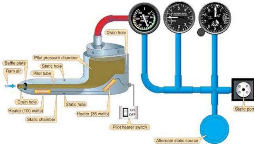
*How are instruments affected when different tubes are clogged?*
