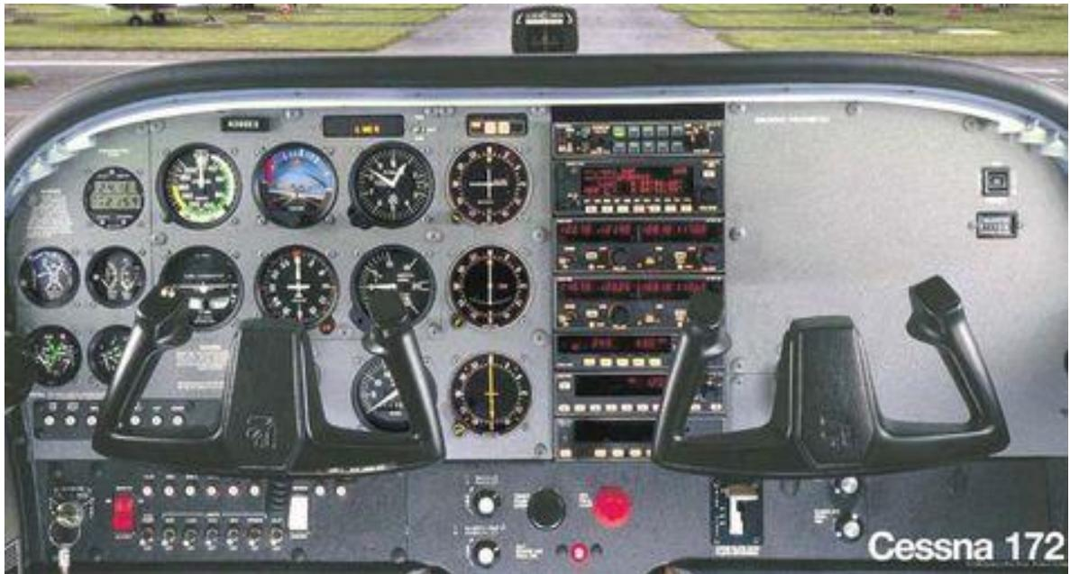
One of the oldest instruments used is the **compass**. However, it is not a very accurate instrument—it is only considered accurate during straight and level flight at a constant airspeed. It has various errors.
