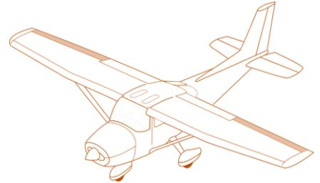
To control the aircraft, we move these primary **control surfaces** to change the [redacted] and [redacted] around the airfoil.
